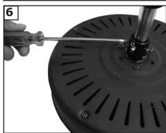
Tighten the 2 Set screws on the Yoke once the downrod is in place. Check motor for shipping stabilizers and remove if present.
